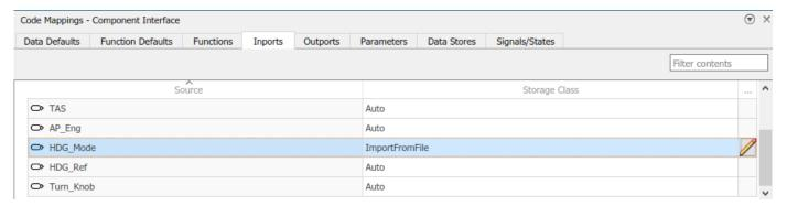
Click the icon and set Identifier to HDG\_Mode and Header File to roll\_heading\_mode.h.
