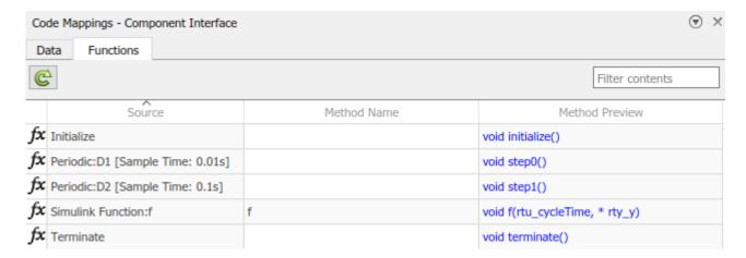
The default name for the initialize class method is initialize, the execution (step) method is step0, and the terminate method is terminate.
