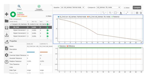
The Simulation Data Inspector shows that the normal mode and SIL mode results match. Comparing the results of normal mode simulation with SIL and PIL simulations can help you verify that the generated application performs as expected.
