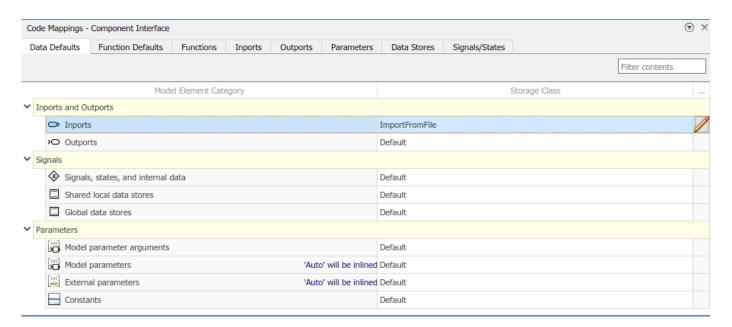
With this setting, the generated code does not define global variables that represent the inport data. Instead, a #include statement includes a header file that declares the input variables. You specify the name of the header file with the Property Inspector.
